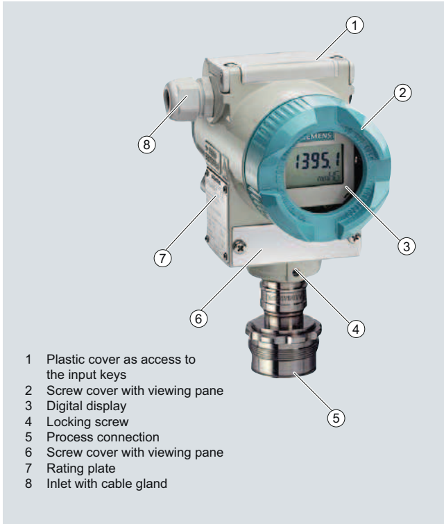
Device front view, SITRANS P DS III
