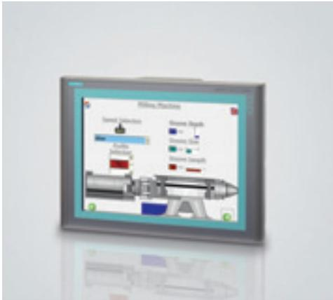
**SIMATIC Multi Panel 377 PRO 15" – a high-performance and robust panel with high openness and expandability**
